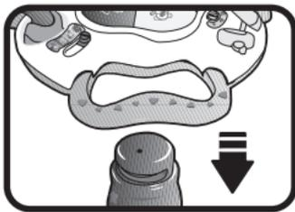
2. To remove the activity panel, pull the release locks located on the bottom of the activity panel away from the center. Pull the activity panel away from the trunk.
